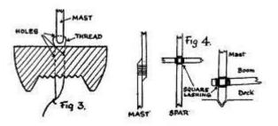
The spars and boom are fixed on with brown thread and a touch of glue.
