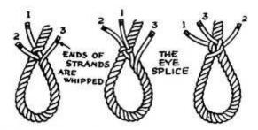
Make sure that each strand is under its own (different) strand. Pull taut and continue the tucks. "Thinning" is done by cutting out about one-third from the underneath side of the strand. After another tuck, another third can be cut away and the spice would then taper nicely.
