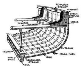
Keel. The lowest part of the boat; it forms the backbone on which the boat is built.
