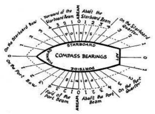
bearings, which is a system of directions taking their names from the ship itself, and is also divided into 32 points.
