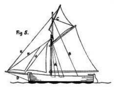
Fig. 5 shows the rigging of a cutter.
