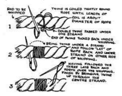
You should take great care of rope, and in this you can set a fine example to other Scouts. If you cut a rope, whip the end as soon as you can, but don't cut it if you can avoid it. Stretch a new rope before using it. Keep your rope dry as far as you can. If it has to pass at any time over a sharp or rough edge, cover the edge with a padding of sacking or canvas or something like. Always coil your rope carefully. (3)
